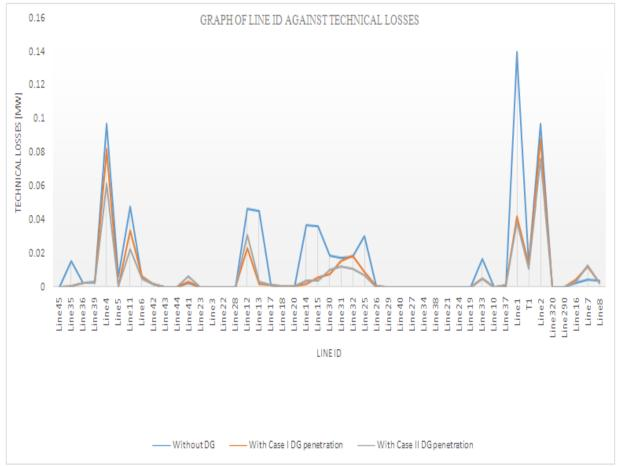
Fig4.3: Graph Comparing Losses without DG, with Case I DG and Case II DG
