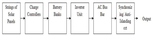
Fig 3.2 Block diagram for interfacing circuit of integrated solar panels
