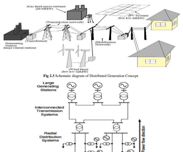
Fig 2.4 Single line diagram of a Distributed Generation concept showing bidirectional power flow
