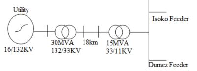
Fig 2.5 Power Supply from Utility to Otovwodo Injection Substation
