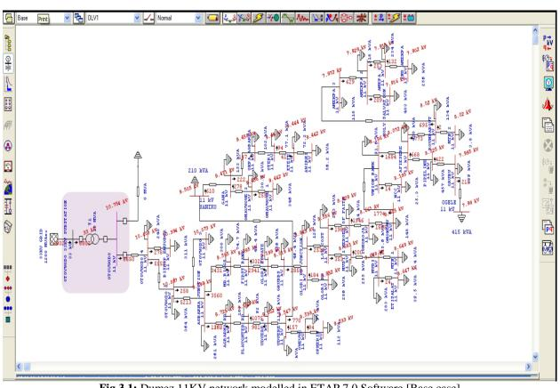
Fig 3.1: Dumez 11KV network modelled in ETAP 7.0 Software [Base case]
