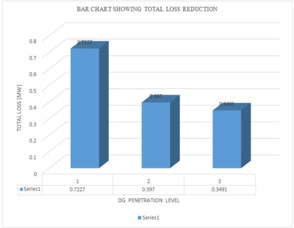
Figure 4.4: Bar chart comparing total Losses without DG, with Case I DG and Case II DG
