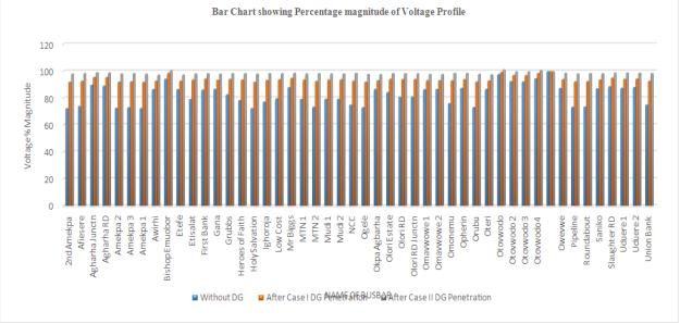
FIGURE 4.8: BAR CHART COMPARING VOLTAGE PROFILE (% MAG) WITHOUT DG, CASE I DG & CASE II DG.
