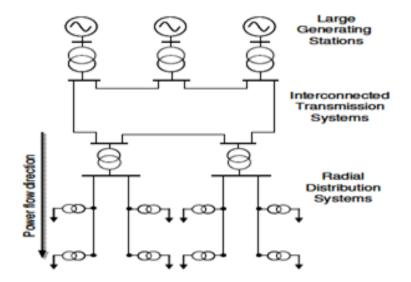
Fig 2.2 Single Line Diagram of a Centralized Concept of Power System Nigeria
